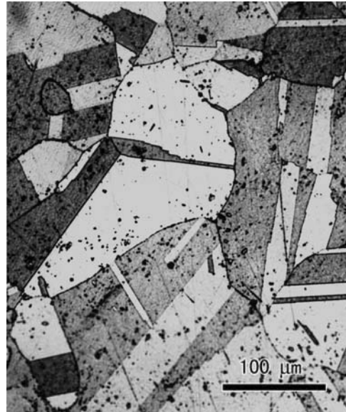
Figure 2 Optical micrograph showing as-heat-treated microstructure of GH4145/SQ alloy.
