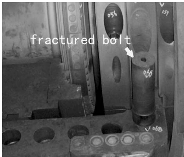
Figure 1 Photograph of a fractured bolt in high-pressure turbine inner cylinder.
